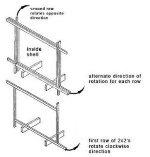
Image 1 - Top: three consecutive layers of 2x2's placed in alternating rotational relationship. First layer rotates counter-clockwise, the second layer rotates clockwise. Bottom: One Layer of 2x2's showing rotational placement. ultimately direct his new innovative approach to structure, material and space.
